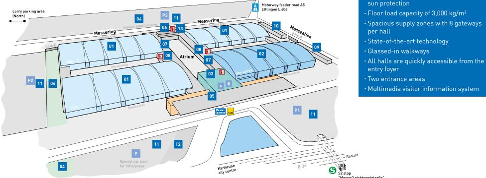
[01] Standard halls: 12,500 m<sup>2</sup> each, column-free, at ground level, variably useable, ample daylight, can be darkened (sun protection), with state-of-the-art service structure, hall height = 17.80 m
